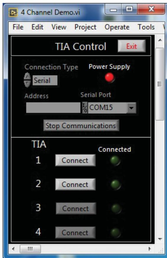
The 4 channel power supply has the capability to detect the presence of any TIAs connected to it. The software will automatically poll the power supply to determine if and where any TIAs are connected. If a TIA is connected to any of the ports, the corresponding controls will enable automatically.
