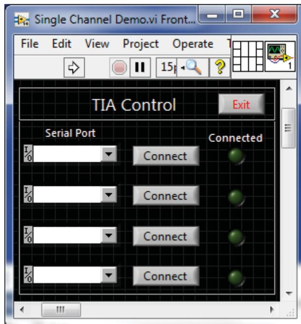
Up to four TIAs with single channel power supplies (Model 3310) can be operated using the demo software. Select the computer serial ports that the TIAs are connected to and press the Connect buttons to connect to the TIA units.
